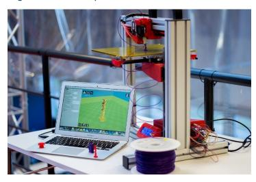
computer-generated model. CAD/CAM systems permit companies to design and manufacture goods faster, more efficiently, and at a lower cost, and they're also effective in helping firms monitor and improve quality. CAD/CAM technology is used in many industries, including the auto industry, electronics, and clothing. If you have ever seen how a 3-D printer works, you have a pretty good idea of how CAM works too.
